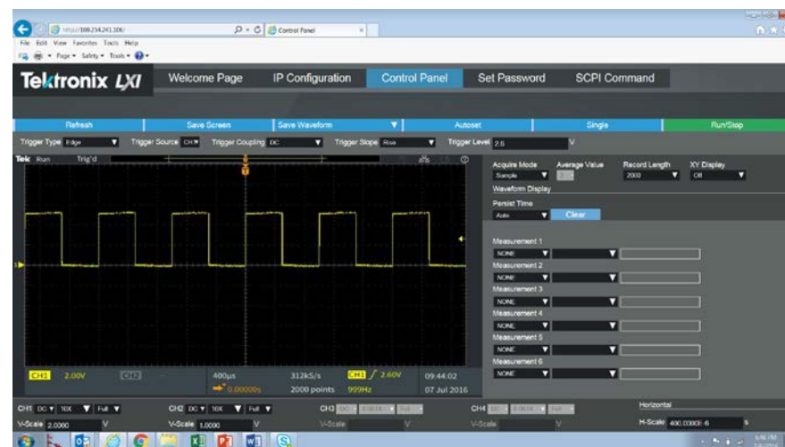
Figure 21. On the PC, the IP has been entered into the address box of the browser, and autoset has been performed remotely
